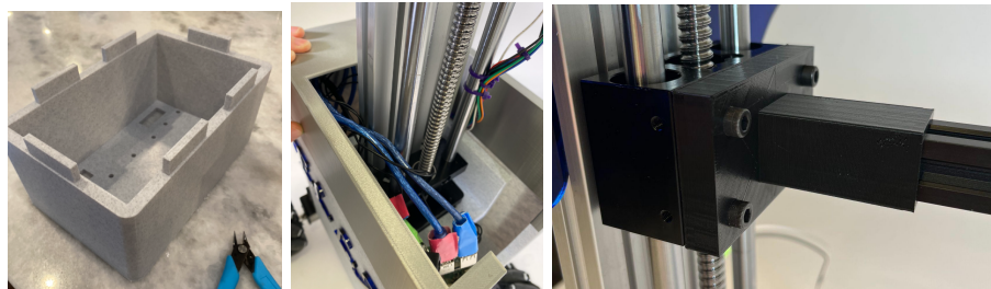
Figure 11-13: 3D Printed Body Piece (1), Electronic Housing View (2), Arm Connector Piece (3)
