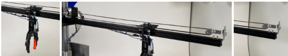
Figure 14-16: Claw/Connector + Color Sensor (1), Pulley System (2-3)
